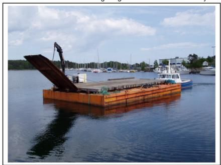
and fine positioning. It's front ramp is used for easy mobilisation of all kinds of equipment.
