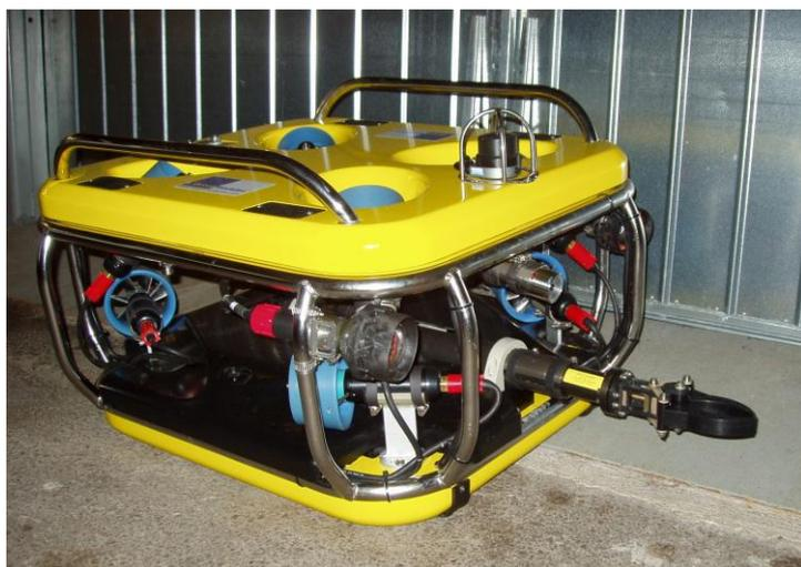
The V8 Sii has a unique configuration of 8 vectored thrusters and state of the art control system allows for precise maneuvering in six degrees of freedom. A positioning system as GPS or UPS (Underwater Positioning System) can be added, providing high accuracy positional data.
